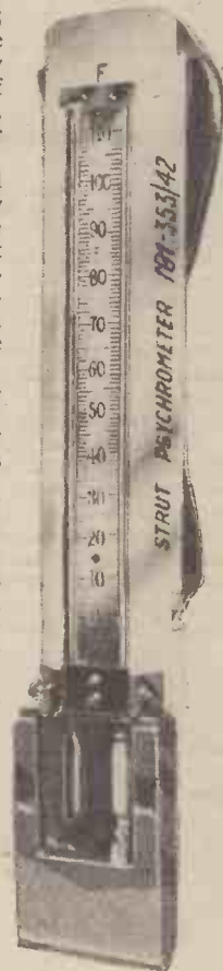
"Strut Psychrometer." An instrument used on meteorological aircraft for recording pressure, temperature, and humidity.—Courtesy of the Meteorological Office, Air Ministry.
